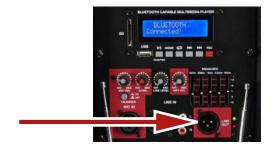
Plug the other end of the cable into the "Line In" of the second speaker
