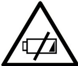
MAKE SURE TO FULLY CHARGE ALL AL7-W UNITS BEFORE STORING THEM. PARTIALLY CHARGED BATTERIES WILL LOOSE CAPACITY.
